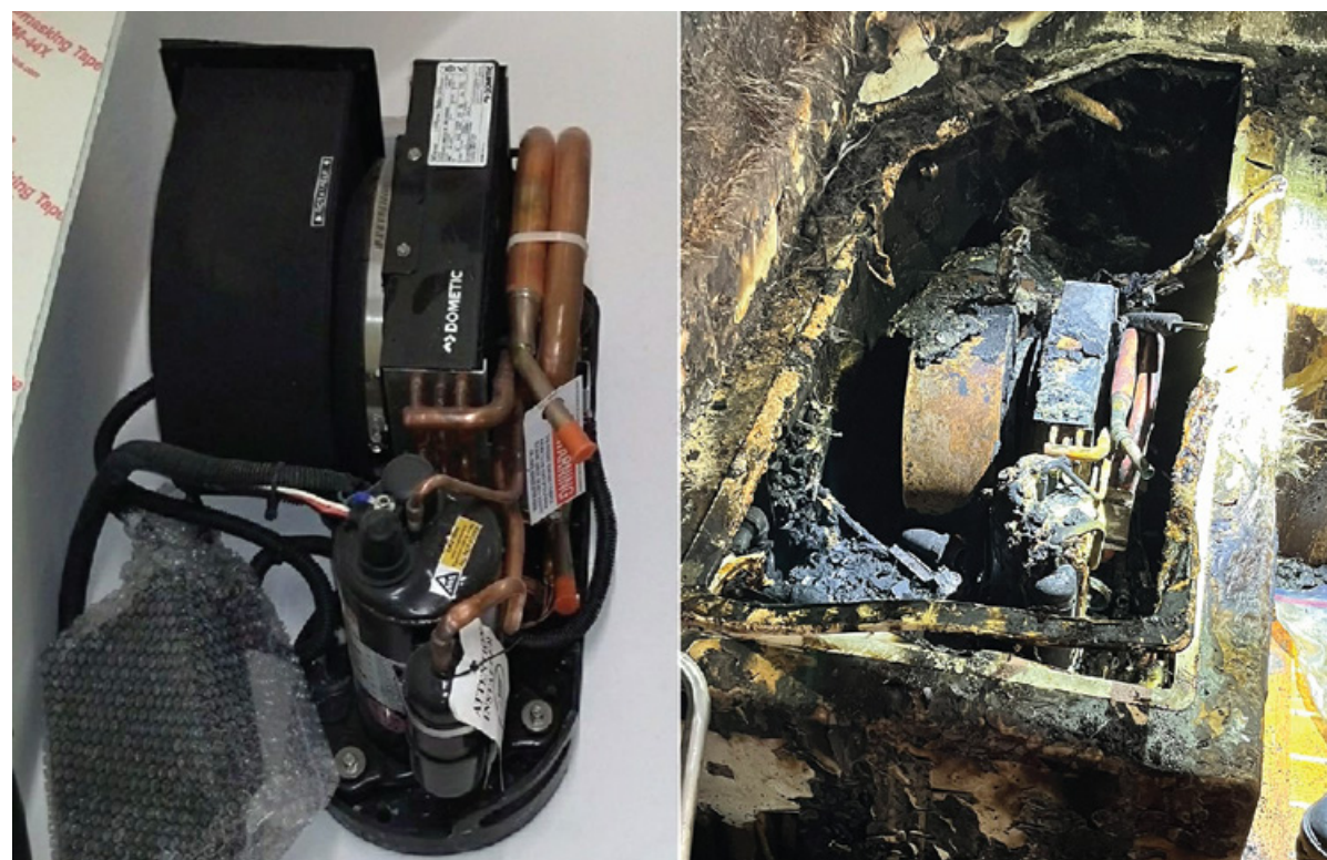
Left to right: Air conditioning unit aboard Whiskey Business in 2019 after vessel construction, and same unit after fire. SOURCE (LEFT): WHISKEY BUSINESS CAPTAIN.
