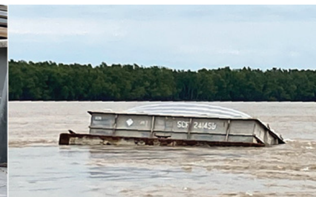
Left to right: Hull indentation on barge SCF14119B and partly sunk barge SCF24145B. SOURCE (RIGHT): COAST GUARD.
