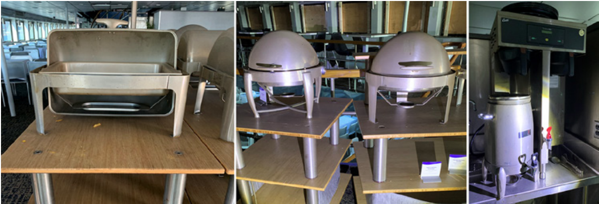
Left to right: Spirit of Boston chafing dishes (with the chafing fuel heating canisters removed) in passenger areas on deck 2 and deck 3 after the fire. Exemplar coffee maker and dispenser used aboard Spirit of Boston with the chafing fuel heating canisters removed from under the dispenser.
