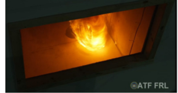
Screenshot of video looking through window of ATF test structure in replicated deck 1 wait station showing flame vectoring and liquified plastic pool (to left of flames) in the area where the plastic glassware rolling cart was located. SOURCE: ATF.
