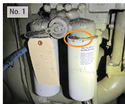
Damage (circled) found on secondary spin-on duplex fuel oil filters from each of the four main engines after the casualty. The no. 1 main engine has a protruding gasket in the direction (outboard) of the no. 2 main engine, and the nos. 2, 3, and 4 main engine filter housings are distorted.
