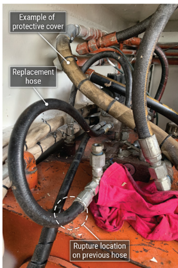
The replacement hydraulic hose, with the location of the rupture on the previous hose circled.
