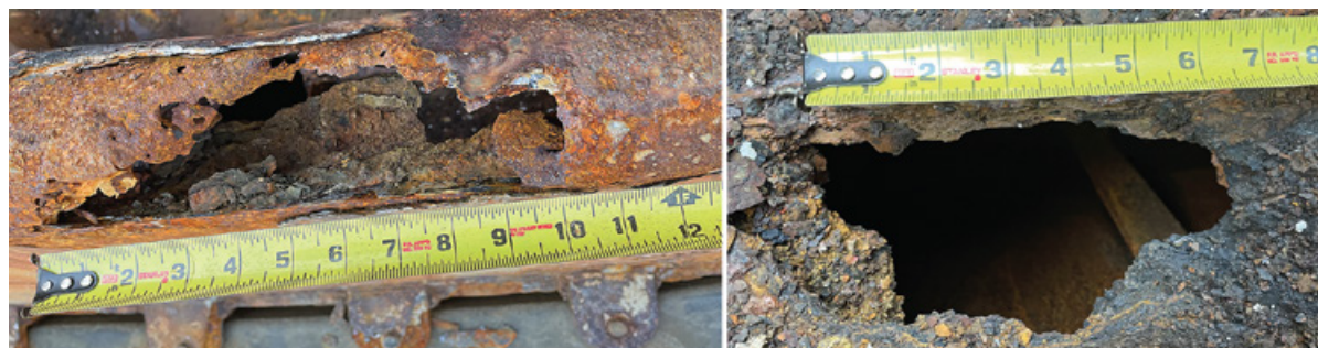
Left to right: Wastage holes on top rail of portside aft bulwarks and in main deck above lazarette within enclosed bulwarks.
