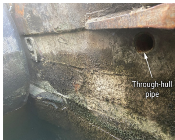
Joanne Marie through-hull pipe for the cofferdam pumps' overboard discharge on the port quarter shown postcasualty.
