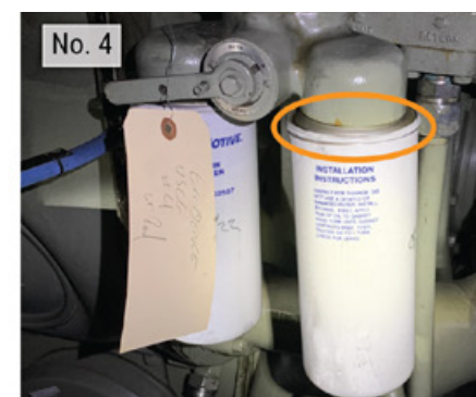
Damage (circled) found on secondary spin-on duplex fuel oil filters from each of the four main engines after the casualty. The no. 1 main engine has a protruding gasket in the direction (outboard) of the no. 2 main engine, and the nos. 2, 3, and 4 main engine filter housings are distorted.
