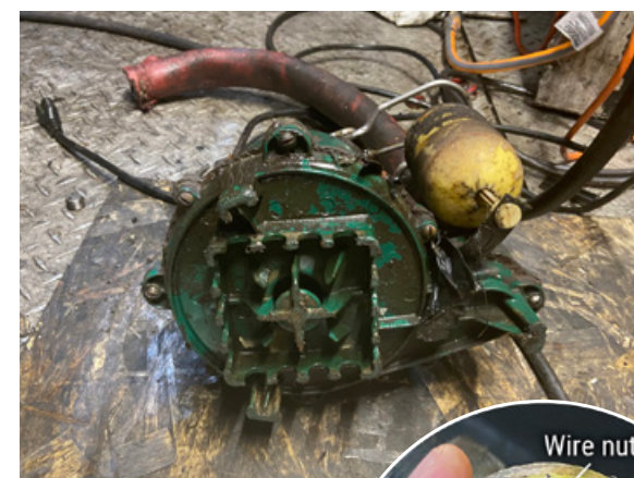
Cofferdam bilge pump with inlet shown with strainer removed. Inset shows associated spring-loaded check valve shown with lodged wire nut.
