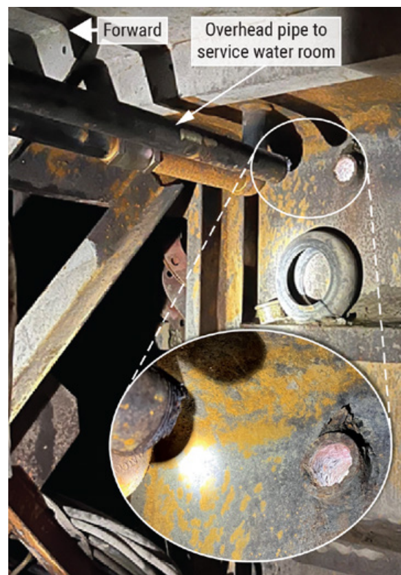
The starboard storage space showing the overhead pipe and the 2-inch through-hull pipe. Inset: The end of the overhead pipe and the unsecured through-hull pipe. SOURCE: COAST GUARD.
