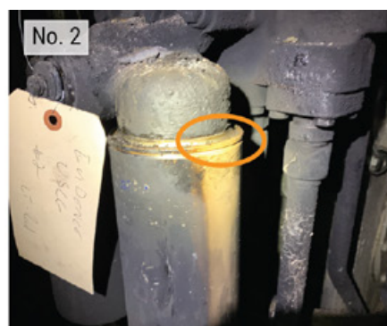
Damage (circled) found on secondary spin-on duplex fuel oil filters from each of the four main engines after the casualty. The no. 1 main engine has a protruding gasket in the direction (outboard) of the no. 2 main engine, and the nos. 2, 3, and 4 main engine filter housings are distorted.
