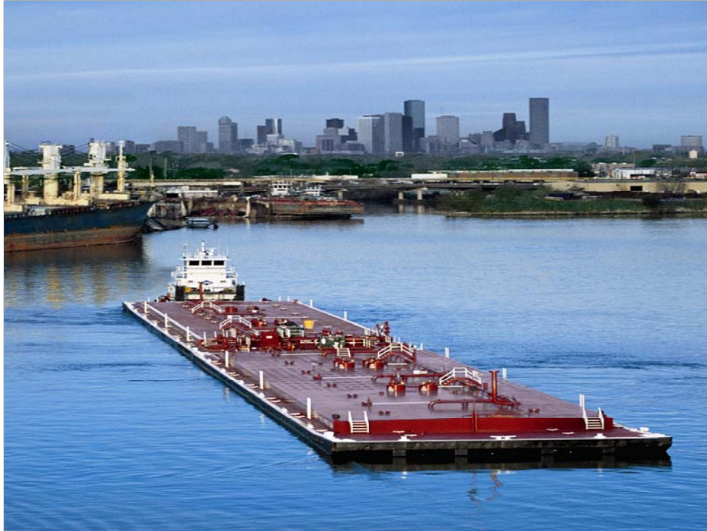
This inland tugboat is pushing a barge full of petroleum or petrochemicals on the inland river system.
