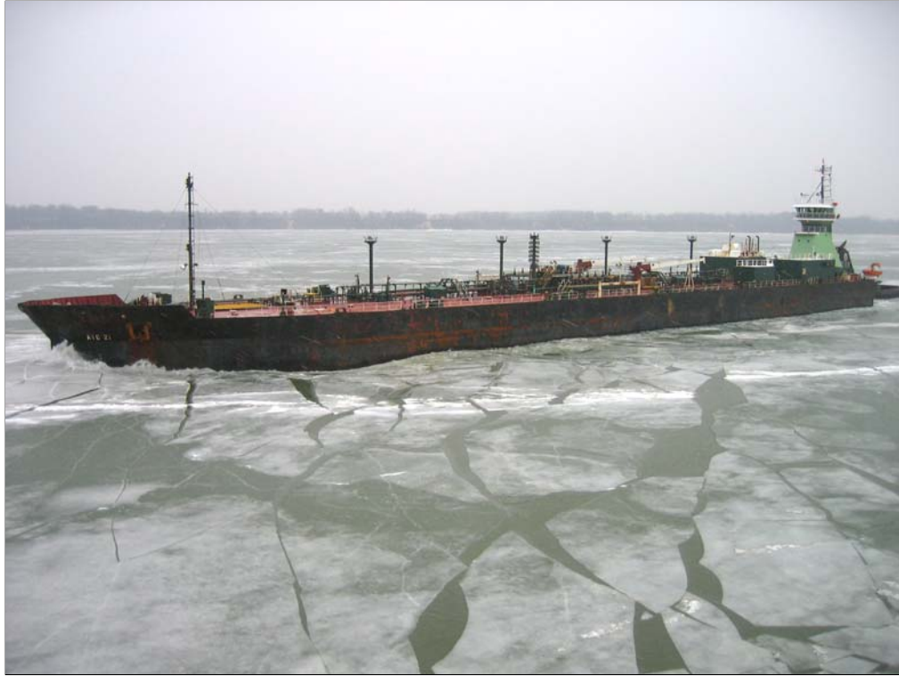
This is an Articulated Tug Barge unit, or ATB, that transports petroleum along the coastline.
