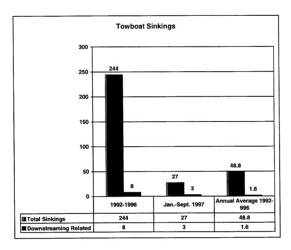
While the number of downstreaming incidents is small, the potential danger to crewmembers involved in a downstreaming sinking is immense. The analysis shows that dating back to 1982, six sinkings resulted in 12 deaths. In two of these cases, all crewmembers were lost, making it difficult to determine causal factors.
